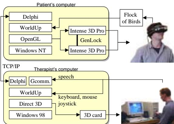
Figure 2: Overview of the Proposed Testbed, Showing How a Second Computer is Connected Using a Delphi DLL.
